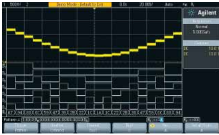
Figure 2. MSOs can capture and display multiple analog and digital signals simultaneously providing an integrated and time-correlated display of multiple waveforms.
